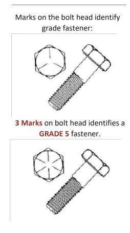
6 Marks on bolt head identifies a GRADE 8 fastener.
