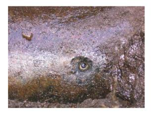
Representative photograph from PHMSA report showing hole in a pipe wall caused by electrical fault (<u>not</u> Olympic Pipeline system)
