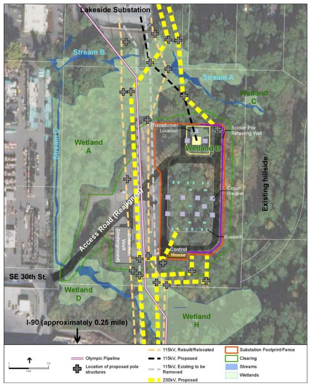
Figure 2-2. Conceptual Site Plan for the New Richards Creek Substation
